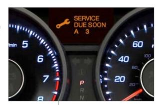
A Honda Maintenance Minder system indicating it is time for a basic (A) service and a transmission fluid (3) service. Honda).
