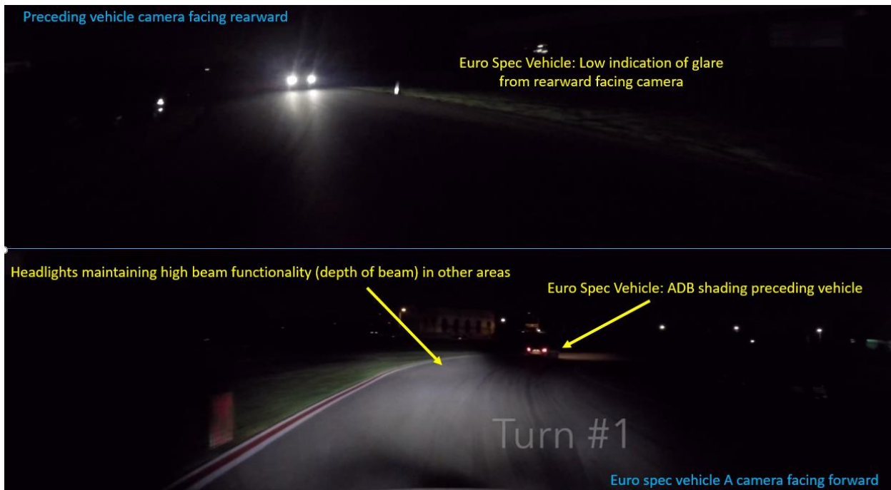
Figure 30: European specification vehicle dynamic testing on closed course
