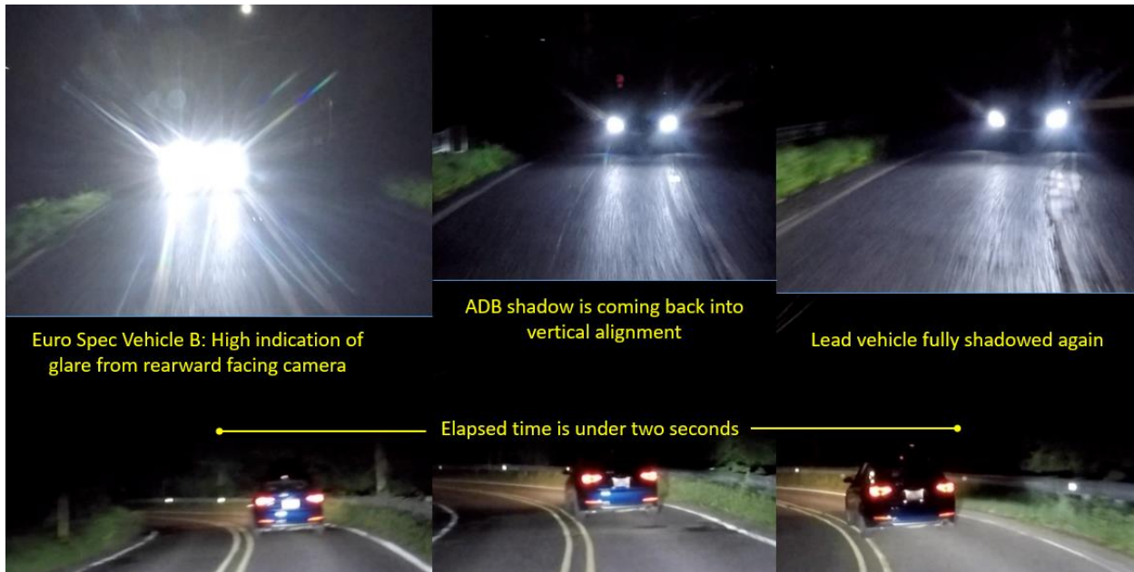
Figure 33: European specification vehicle losing vertical alignment of ADB shadow and correcting
