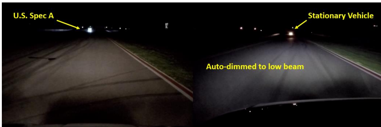
Figure 26: U.S. Specification Mfg. 2 Glare Drive-by with Headlamps Auto-dimmed to Low Beam
