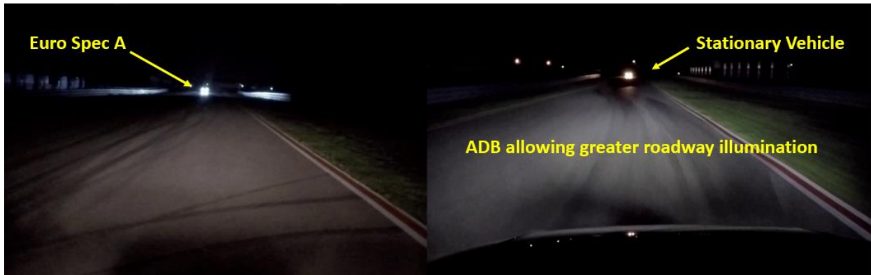
Figure 27: European Specification Mfg. 2 Glare Drive-By with Headlamps in ADB mode
