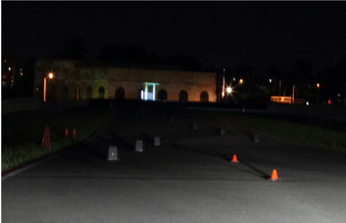
Figure 12: Target illumination view from U.S. specification mfg. 1, low beam
