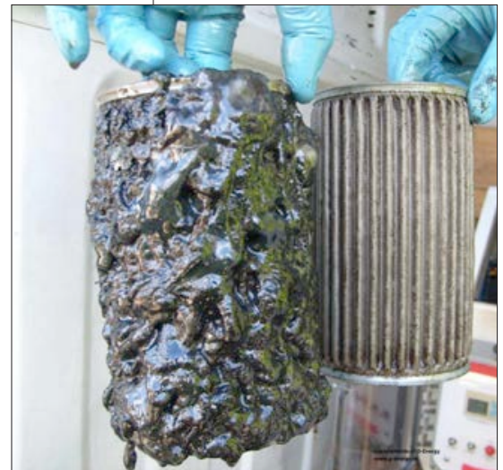
A diesel fuel filter plugged as a result of microbial growth.
