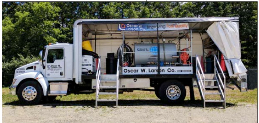
A service truck equipped for fuel storage tank cleaning and fuel polishing. (Image: Oscar W. Larson Co.)
