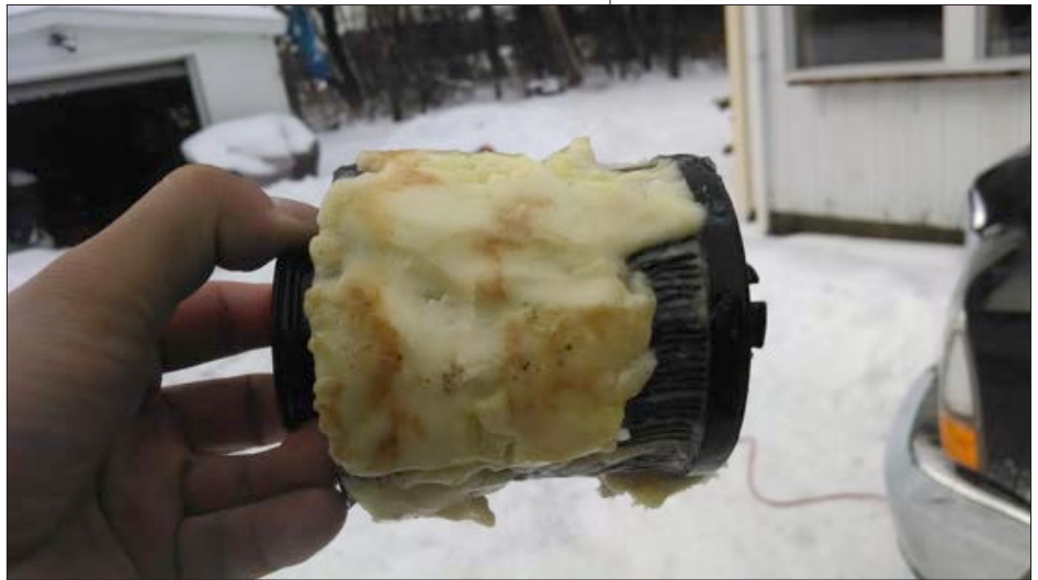
A fuel filter covered with paraffin wax from gelled diesel fuel. (Image: Advanced Fuel Solutions, Inc.)
