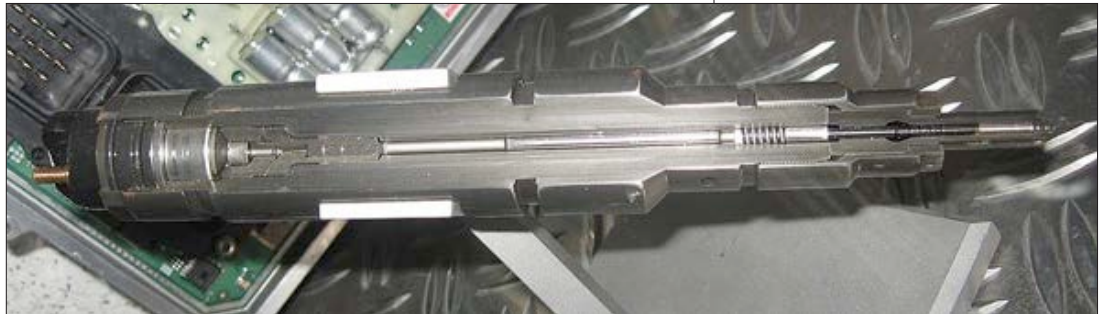
A cutaway view of a piezoelectric diesel fuel injector whose tight tolerances rely on fuel lubricity to prevent damage. (Image: L. Kenzel, GNU FDL 1.2 or later)
